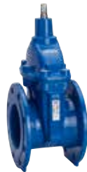
Series 06/84 Flanged gate valve Short face to face DIN F4 NBR wedge AISI 316 stem Ductile iron DN40-600 and 800 From DN450 with ISO top flange
