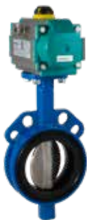
Series 820/00 Centric butterfly valve with loose NBR liner Wafer Ductile iron DN25-1000 With any type of actuation
