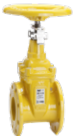
Series 06/59 Flanged gate valve with position indicator Short DIN F4 DN50-400 PN10/16 Ductile iron With external epoxy coating
