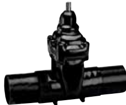
Series 46/70 Gate valve with long spigot ends DN50-600 PN16 GP240GH With external PUR coating
