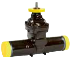
Series 46/78 Gate valve with long spigot ends and ISO top flange DN50-400 PN16 GP240GH With external PUR coating
