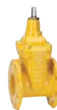
Series 06/70 Flanged gate valve Short DIN F4 DN40-600 PN10/16 Ductile iron With external epoxy coating
