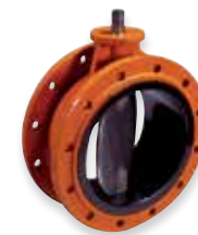
Series 75/20 Double flanged short butterfly valve, centric with fixed liner DN50-600 PN10/16 Ductile iron
